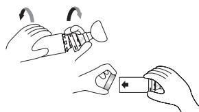
Remove the **Backpiece**, mask adapter and mask only. DO NOT attempt to remove any other parts.
