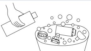
Soak all parts for 15 minutes in a mild solution of liquid dish detergent and lukewarm clean water. Agitate gently.
